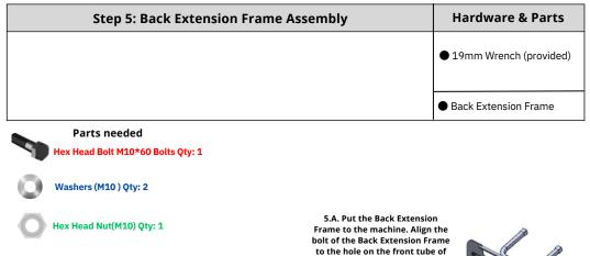
5.B. Push through the Back Extension Frame until the bolt sticks out, put on the washer and the nut then hand tighten. Once done, fully tighten using wrench.
