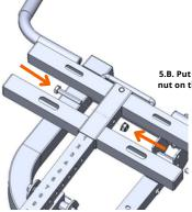
5.B. Put the bolt on the middle hole then washer and the nut on the other side then hand tighten. Once done, fully tighten using wrenches.
